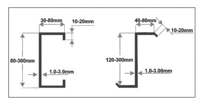
A complete range of structural C and Z purlins for industrial buildings, garages, verandahs, and carports, in fact anywhere that strong, reliable steel framing is required. Manufactured from quality galvanised steel, this is a fully integrated system allowing for flexible design options.
